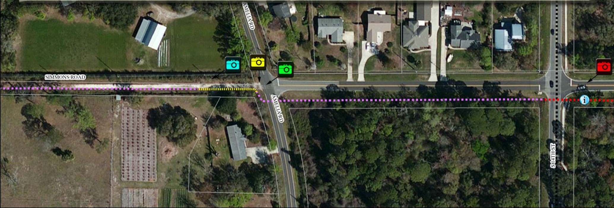
THE TRANSITION FROM THE AMELIA ROAD ROW TO THE SIMMONS ROAD ROW ON THE WEST SIDE OF AMELIA ROAD WILL REQUIRE THE REPLACEMENT AND EXTENTION OF THE CULVERT RUNNING BENEATH THE UNPAVED PORTION OF SIMMONS ROAD.
